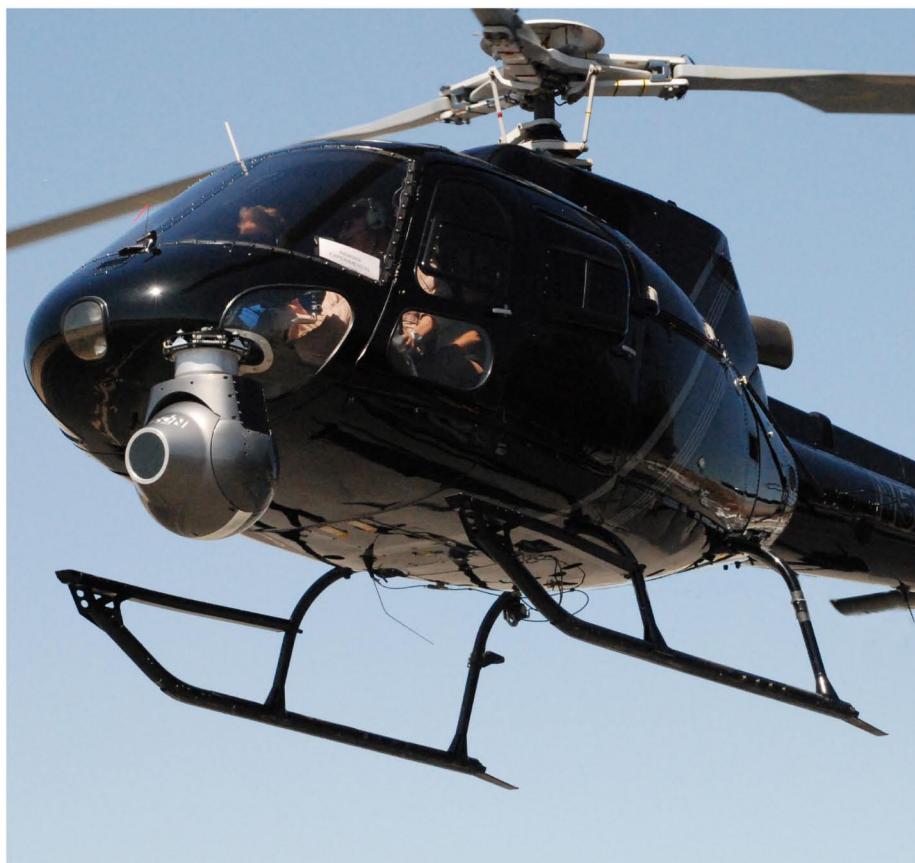
Figure 1. Left Front Mount and Typical Payload Installation
